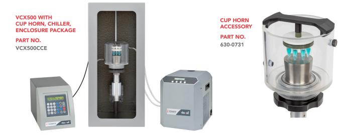
The cup horn is attached to the converter in place of a probe, and filled with water. Microtubes containing samples are placed inside using specially designed tube holders. Ultrasonic energy is transferred through the water and into the sample tubes. Multiple tube holders are available for various size tubes and vessels. Both types of 1.5mL tube holders shown below are included.
